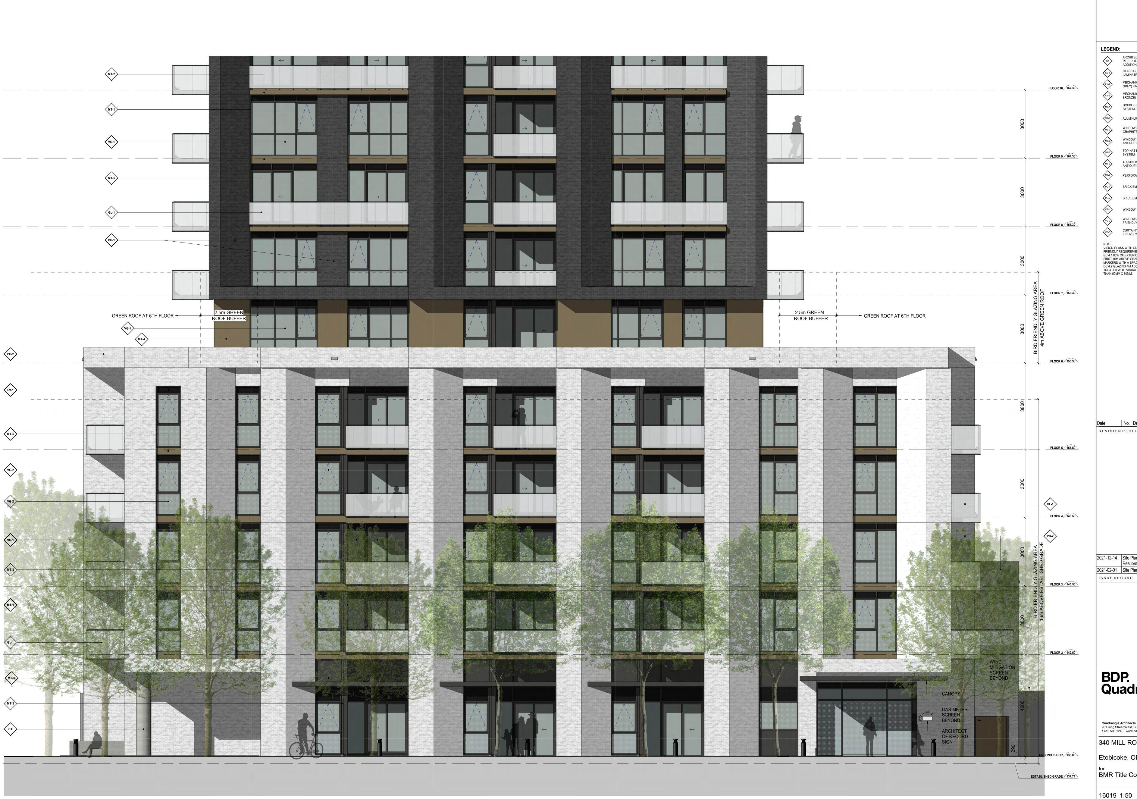
ARCHITECTURALLY EXPOSED CONCRETE -REFER TO STRUCT SPECIFICATIONS FOR ADDITIONAL REQUIREMENTS GLASS GUARD - HEAT-STRENGTHENED LAMINATED GLASS WITH COLOUR INTERLAYER MECHANICAL LOUVRE WITH MT-1 (GRAPHITE GREY) FINISH MECHANICAL LOUVRE WITH MT-2 (ANTIQUE BRONZE) FINISH
