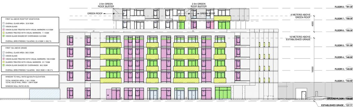
4 BIRD-FRIENDLY GLAZING CALCULATIONS - SOUTH ELEVATION
