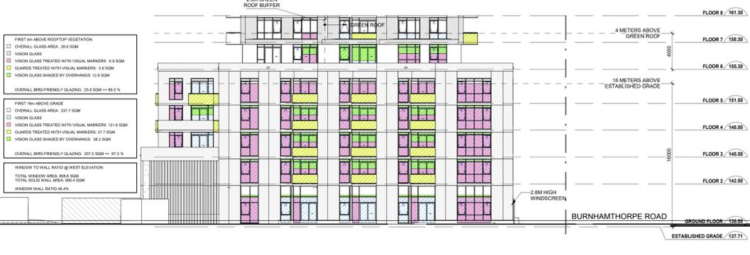
4 BIRD-FRIENDLY GLAZING CALCULATIONS - WEST ELEVATION
