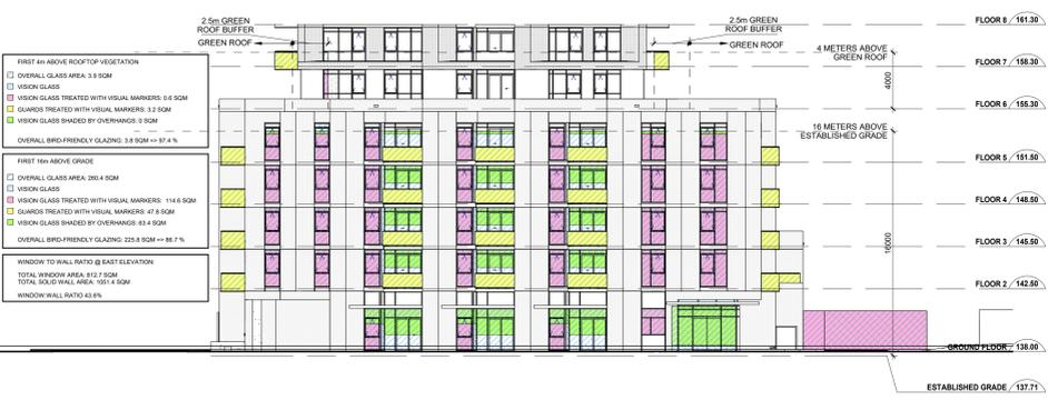
3 BIRD-FRIENDLY GLAZING CALCULATIONS - EAST ELEVATION
