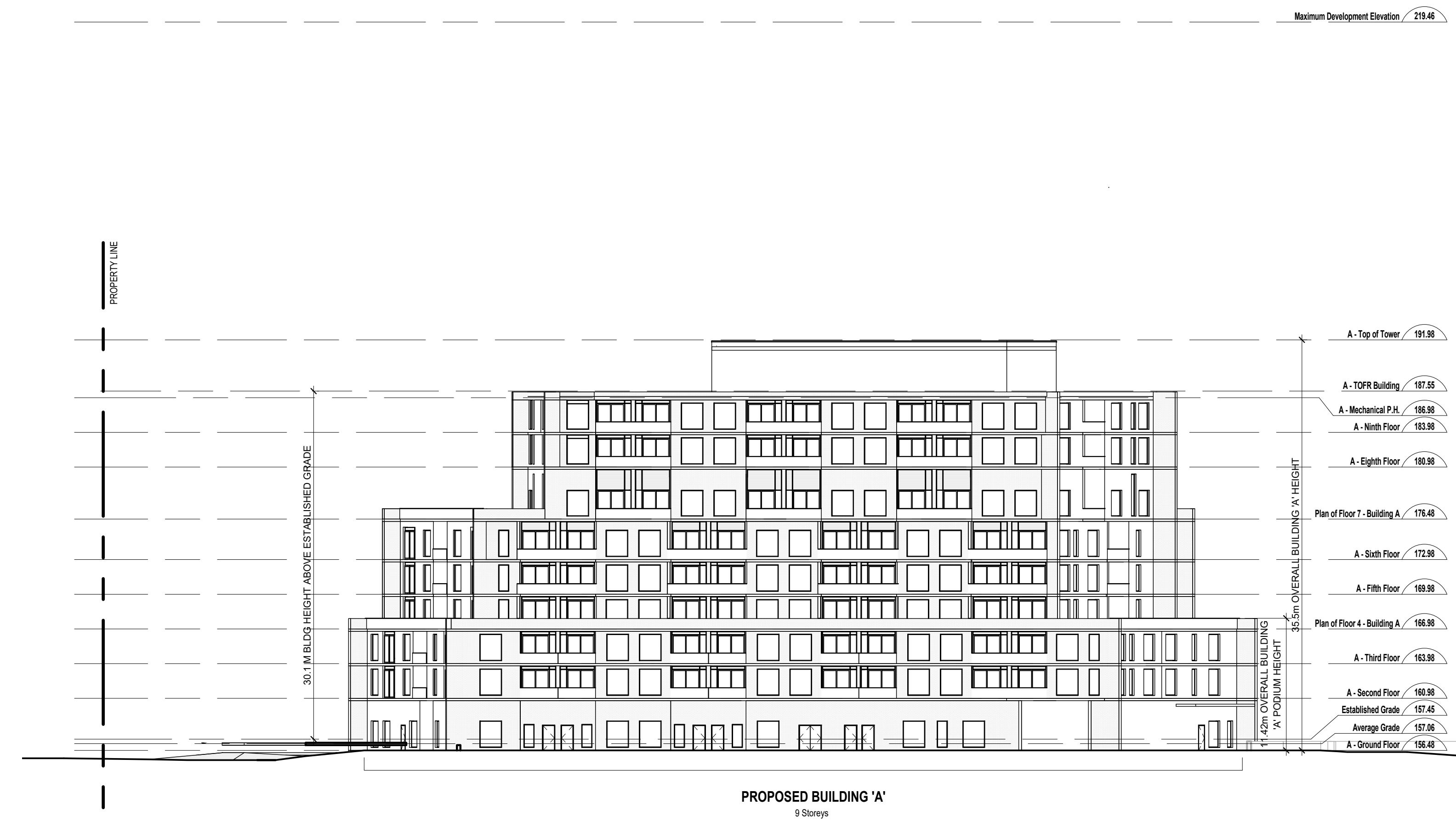
2 PROPOSED RESIDENTIAL BUILDING 'A' EAST ELEVATION
